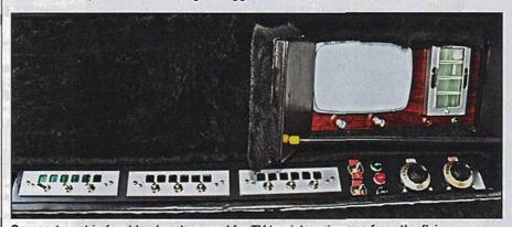
Compartment in front backrest opened for TV to pick up images from the flying scanner. Two large rotating knobs were non functional. Indicator lights and switches to the left were a master power function and for deploying the rams that attached to fixtures in the garage floor. The three big switch consoles controlled all the special features—oil slick, front and rear rocket doors, decklid scanner trap doors, scanner platform elevator, rear brooms, headlight and license plate rotation, etc.
