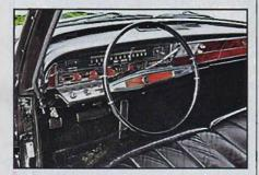
Exterior of dash is stock, save for the speaker connected to the internal PA system and for radio signals. The wheel is a non-tilter, and there were no seatbelts or spare tire. Upholstery is the standard black leather.
