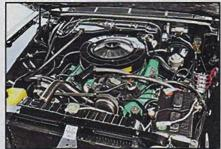
Original 11K-mile 413 has been freshened and fitted with a Hughes cam for more torque. Engine compartment has been detailed. Car came with all its assembly line belts, hoses, clamps and wires that were replaced for reliability, but were stashed away.
